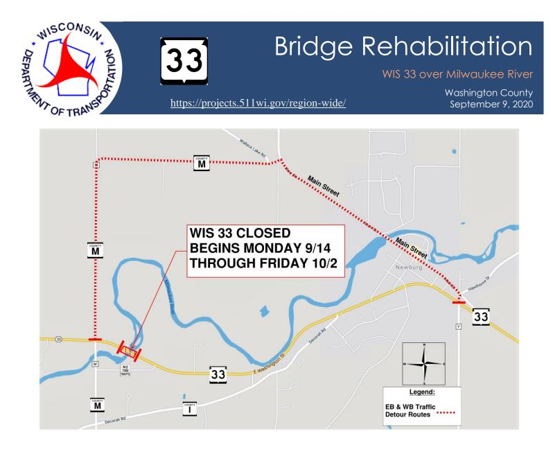
The Wisconsin Department of Transportation will be closing WIS 33 over the Milwaukee River on Monday September 14<sup>th</sup> for approximately three weeks to complete bridge deck repairs. The Bridge deck will be repaired and overlaid. Bridge approach pavement will be overlaid.
