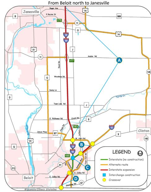
A I-39/90 northbound: Reconstruction and expansion from Hart Road near Beloit north to the I-39/90 and US 14 interchange (Exit 171B) in Janesville. **Construction: fall 2017 – spring 2020**
