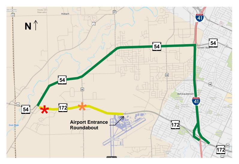
WIS 172 Resurfacing Work Zone (open to traffic with temporary lane closures and flagging operations)
