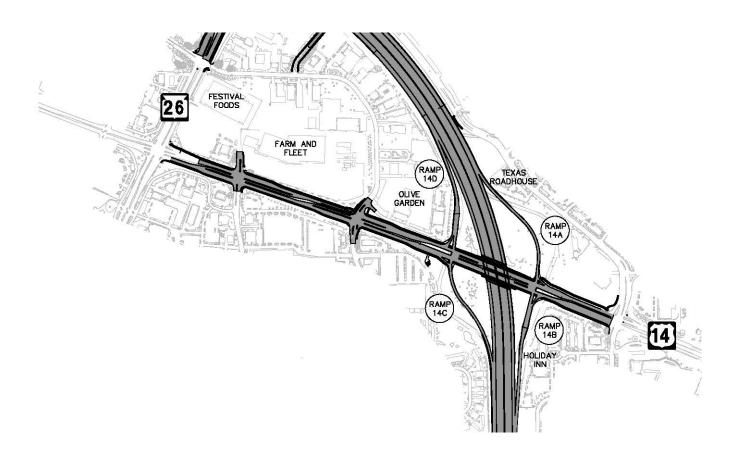
All US 14 ramps will be impacted by the re-construction of US 14. During construction the intersections will be staged to a point where it requires the closure of each ramp to complete the final intersection configuration. The closure is needed to complete the required earthwork, gravel, concrete paving, concrete curing, pavement marking, signing, and traffic signal construction. None of the ramps will be closed concurrently.
