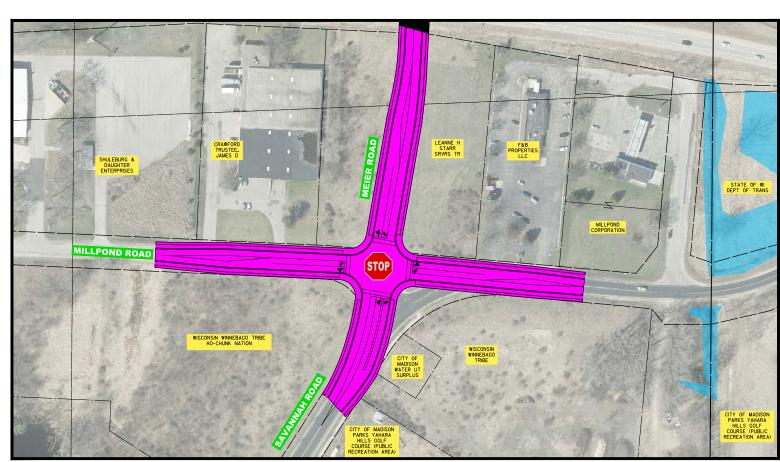
CONCEPTUAL STOP CONTROL INTERSECTION LAYOUT (2-WAY OR 4-WAY STOP)
