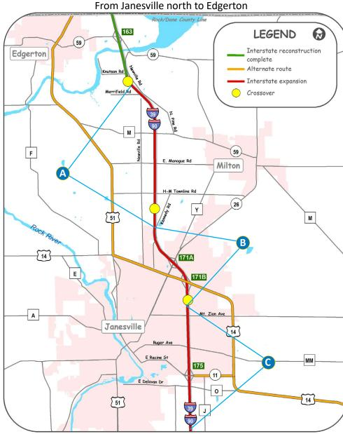
A I-39/90 southbound: Reconstruction and expansion for about six miles of Interstate from Kennedy Road, north of the WIS 26 interchange (Exit 171A), to just south of the Rock River bridges near Edgerton.
